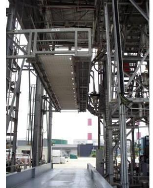
The system is ideal for loading on weighbridges as the platform only has contact with the tanker via limit switches.
