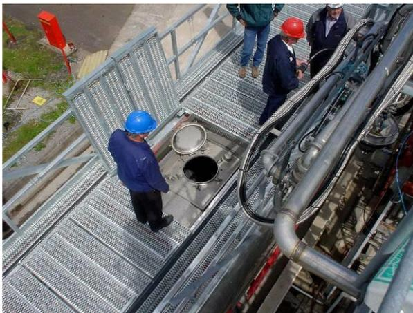
Full and safe access to the tanker manholes, without risk of falling or reliance on tanker walkways.
