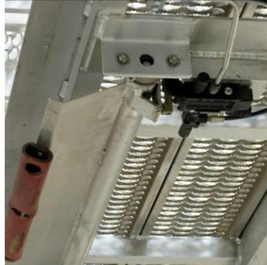
The system is supplied with Tanker Detection Switches that stop the downward movement when the full length detection flaps contact the tanker
